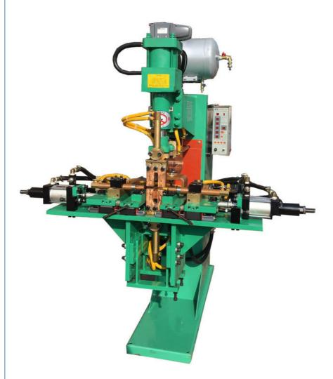
The push cylinder of this machine is inside the machine, which is an internal T-spot welder
