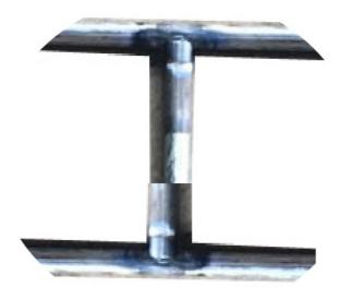
T-type spot welding machine mainly uses T-type butt joint of iron wire process products, metal basket, hardware parts, iron wire on hook and iron pipe.
