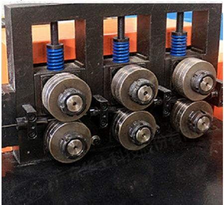
3. The straightening system adopts multi wheel straight forward straightening, with high speed and no distortion.
